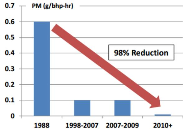
The above image demonstrates how far diesel emission control technology has come in just the past 20 years. Most amazing, is while U.S. emission standard have fallen dramatically, [recent testing](#) shows that the engines are actually outperforming the standards by a wide margin.
