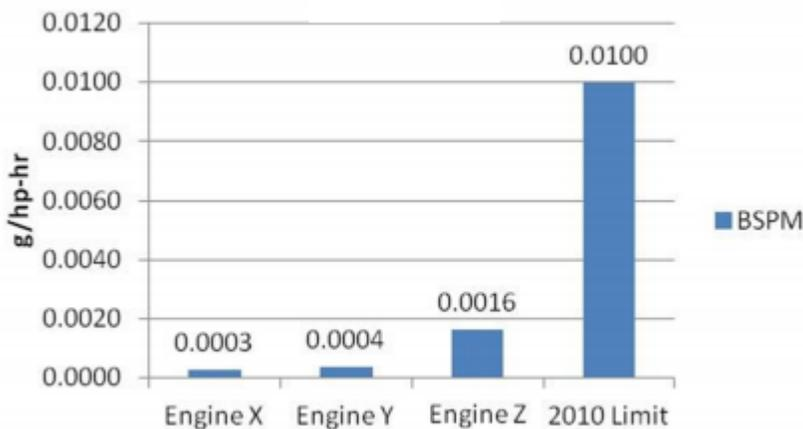
Diesel particulate matter has been virtually eliminated. Note that while the emission standard has fallen by 98% since 1988, actual emissions have fallen by 99.9%.
