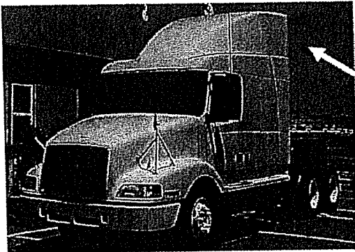
Figure 2: Baseline Assumption: "Aero Cab" Tractor with Roof Fairing
