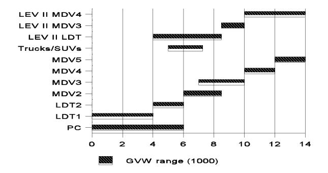
both the LDT2 or MDV2 categories because the higher payload will cause some of the vehicles to be placed in the MDV2 category. Payloads can also vary between vehicles in the MDV2 and MDV3 categories causing the same model to be certified in both categories because of payload differences. This figure also includes the proposed LEV II vehicle classes that will be discussed later in this report.
