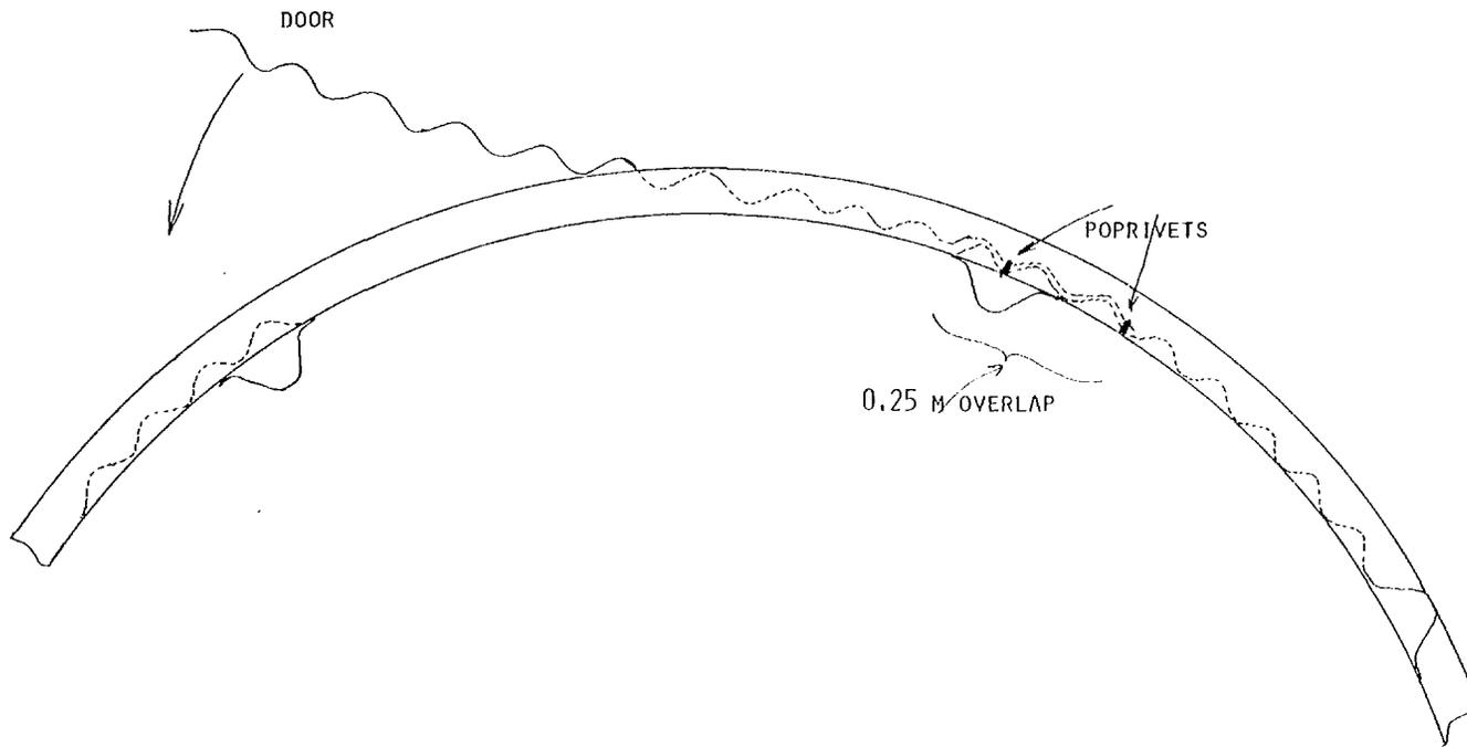
Figure A-4. Design for corrugated fiberglass door for orange open top field chamber.
