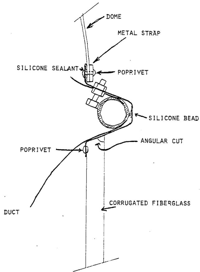
Figure A-5. Design for attaching dome panels and base panels to upper rolled galvanized metal hoop of orange open top field chamber.
