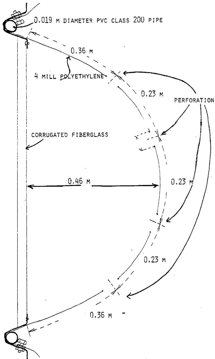
Figure A-6. Design for attaching vinyl plastic duct to upper and lower galvanized metal hoops of the orange open top field chamber.
