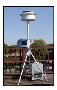
We chose the Beta Attenuation Monitor (BAM) for use in California and have installed monitors at 103 sites. The U.S. Environmental Protection Agency (U.S. EPA) designated certain models of the continuous monitors as Federal Equivalent Monitors (FEM). They are considered to provide equivalent data to the Federal Reference Monitors and can therefore be used to determine compliance with federal standards. California has deployed 59 of these FEM monitors.
