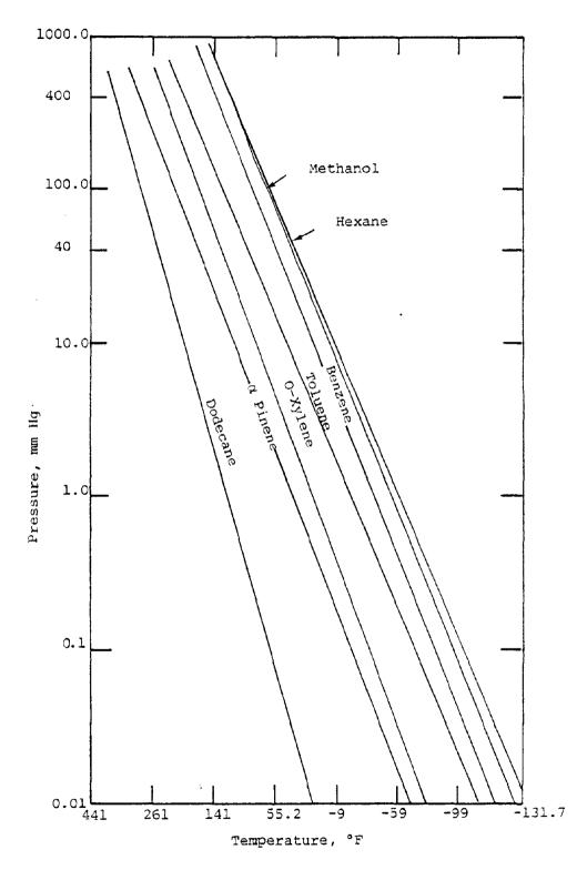
Figure 4-14. Vapor pressures of organic solvents versus temperature. KVB 5804-714
