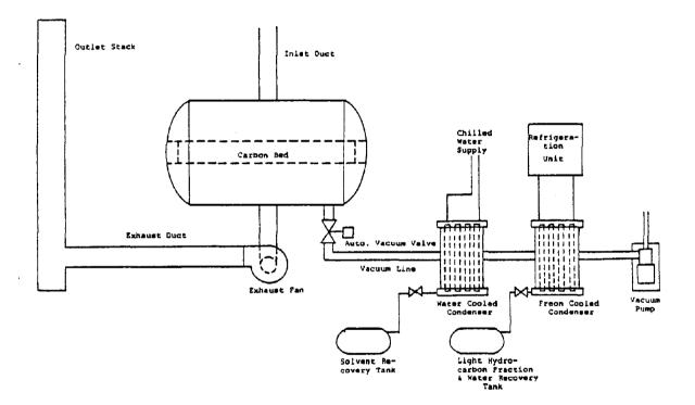
The tank to be regenerated is removed from the adsorbate stream by automatically closing the process vacuum valves at the top and bottom of the tank. Then, a smaller vacuum valve is automatically opened connecting the
