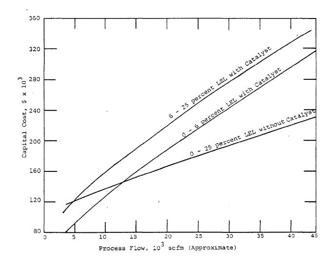
Figure 4-35. Capital cost for direct flame and catalytic afterburners with primary heat recovery (70 - 300 °F process gas inlet) (1976 prices) Case 2 (Ref. 4-2).
