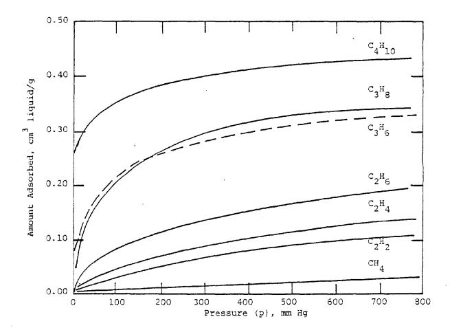
Figure 4-1. Adsorption isotherms of hydrocarbon vapors (amount adsorbed at pressure, p, on type Columbia L carbon at 100 °F, Ref. 4-1).
