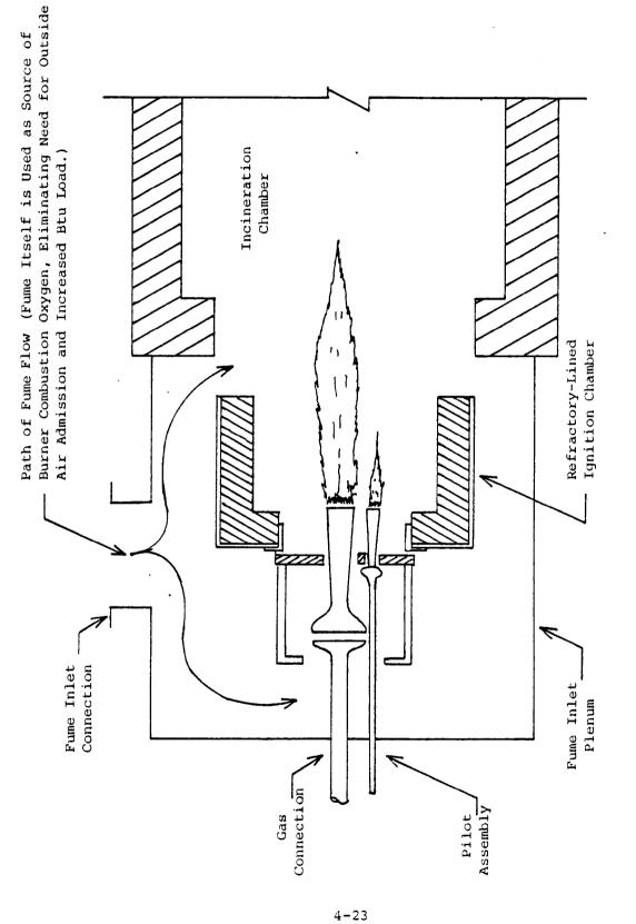
Figure 4-7. Typical burner and chamber arrangement used in direct-flame incinerator.
