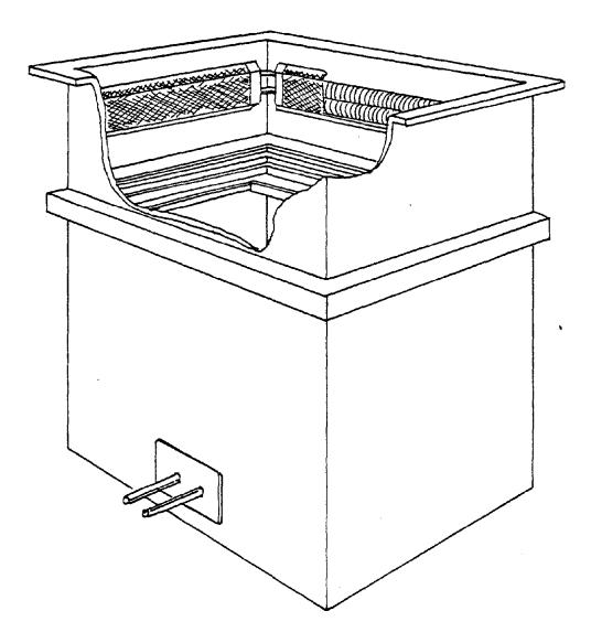
Figure 4-17. Refrigerated freeboard chiller.
