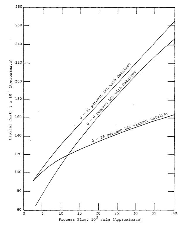
Figure 4-30. Capital cost for direct flame and catalytic afterburners without heat recovery (70 - 300 °F process gas inlet) Case 1 (1976 prices) (Ref. 4-2).
