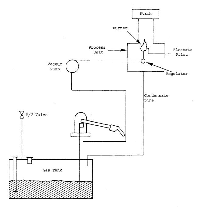
Figure 4-21. Hasselmann thermal oxidation system for control of automobile refueling vapors.
