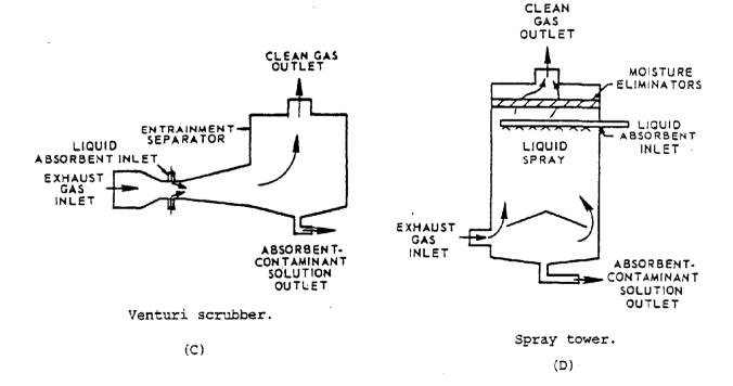
Figure 4-18. Types of absorption systems.
