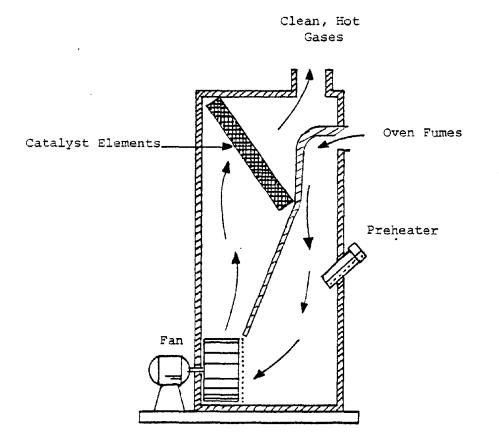
Figure 4-12. Schematic diagram of catalytic afterburner using torch-type preheat burner with flow of preheater waste stream through fan to promote mixing (Ref. 4-1).
