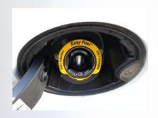
1. Capless fill pipes with open drain path
