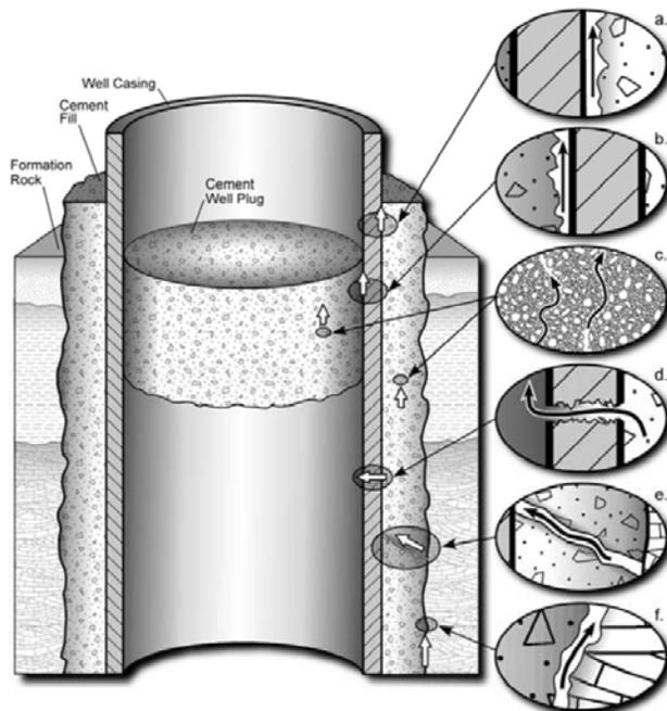
**Figure 1:** Schematic of possible leakage pathways along a well (a) between cement and outside of casing, (b) between cement and inside of casing, (c) through cement, (d) through casing, (e) in cement fractures, (f) between cement and rock.<sup>25</sup>
