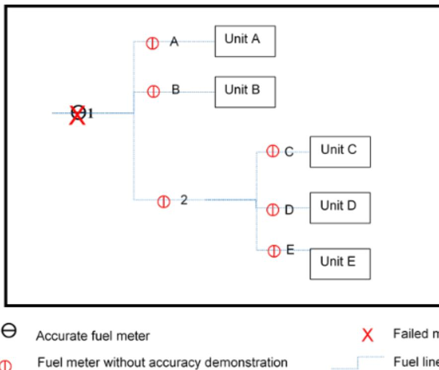
Description of scenario: In this scenario, none of the meters used to monitor fuel consumption to individual units meet the accuracy requirements, and there is no valid upstream meter data available.
