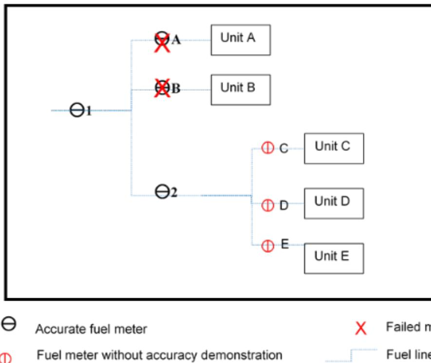
Description of scenario: In this scenario, Meters 1 and 2 have met all accuracy requirements or are financial transaction meters. Meters A and B have failed the accuracy requirements, and the accuracy of Meters C, D, and E is unknown.
