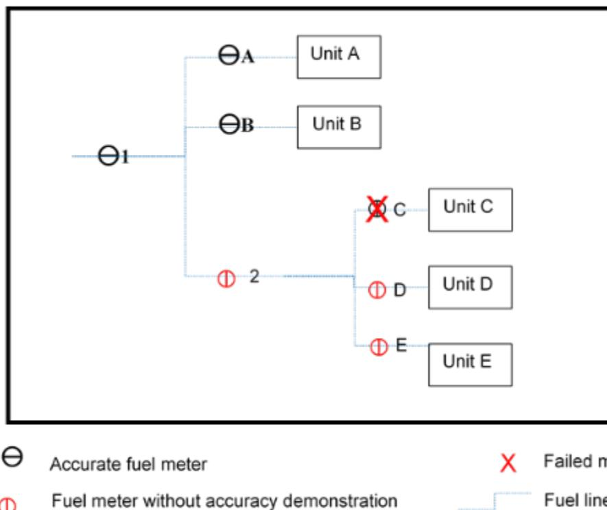
Description of scenario: In this scenario, the facility-level meter is accurate, but a downstream meter does not have an accuracy determination, and a unit meter failed.
