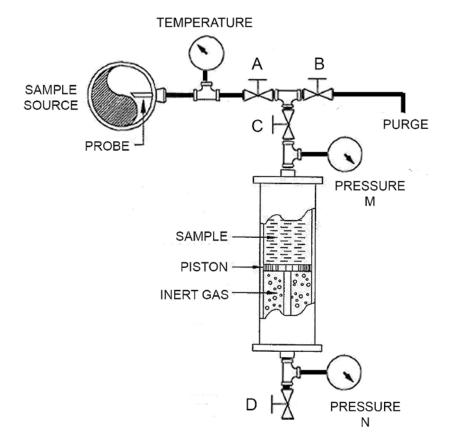
Figure 3: Piston Cylinder Sampling Train
