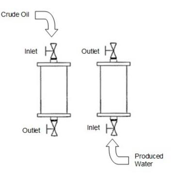
Figure 2: Double Valve Cylinder Orientation
