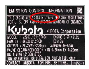
Other current-tier emissions labels just indicate the model year of the engine and require the reader to look up the tier standard met. An example of such a current-tier engine emissions compliance statement is: THIS ENGINE COMPLIES WITH U.S.EPA AND CALIFORNIA REGULATIONS FOR 2009 M.Y. NONROAD AND STATIONARY/OFF-ROAD DIESEL ENGINES." The picture to the right shows an example of such an emissions label. The power rating of the engine in this picture shows 11.3 kW, which is 15.2 horsepower
