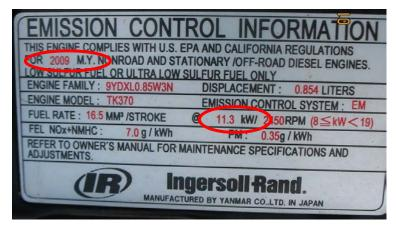
(note that 1 kW equals 1.341 hp). Table 1, above, indicates the years that each tier standard was in effect. By examination of Table 1, a less than 25 horsepower, model year 2009 engine was required to meet Tier 4.
