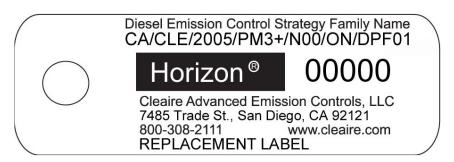
The following sample label is permanently attached to the diesel particulate filter:
