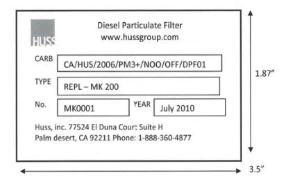
CARB label is metal and should be displayed on the engine and the filter.
