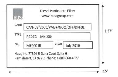
CARB label is metal and should be displayed on the engine and the filter.
