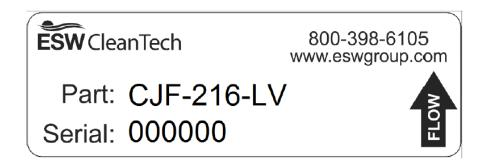
The following sample label is permanently attached to the lean NOx catalyst:
