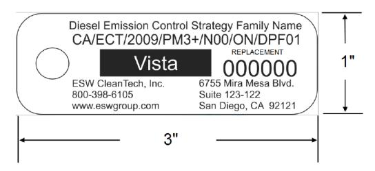
The following sample label is permanently attached to the diesel particulate filter:
