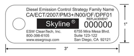
The following is an illustration of the label that is permanently attached to the diesel particulate filter:
