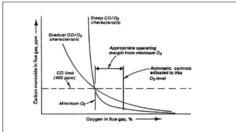
**Figure 1** Oxygen/CO Characteristic Curve
