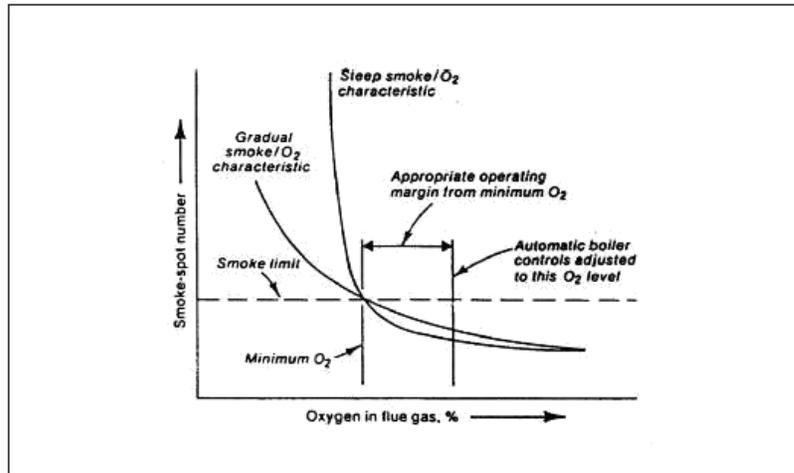
**Figure 2** Oxygen/Smoke Characteristic Curve
