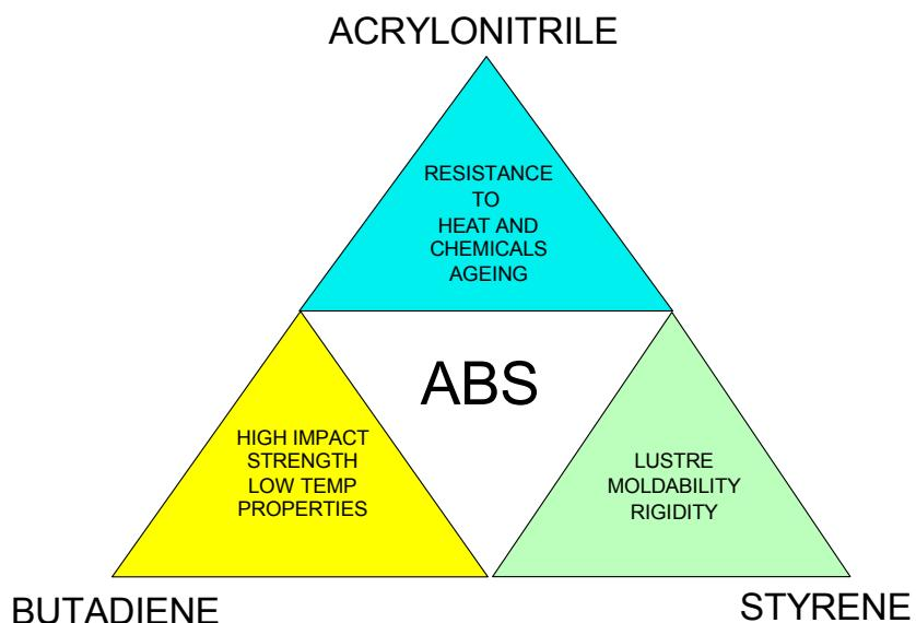
These properties make ABS suitable for injection moulding, extrusion, blow and foam moulding and thermoforming. It can be easily processed through machined, bored turned, milled, sawed, die cut, routed, filed, sanded, ground buffed and polished. ABS may be pigmented and though they are usually translucent to opaque, they may be produced in transparent grades.
