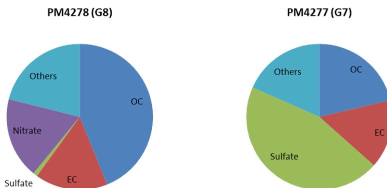
**Figure 1. PM composition comparison: PM4278 (G8, 2010 engines) vs. PM4277 (G7, 2007 engines)**
