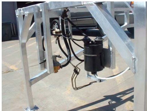
Figure 4. Canister and Controls Mounting
