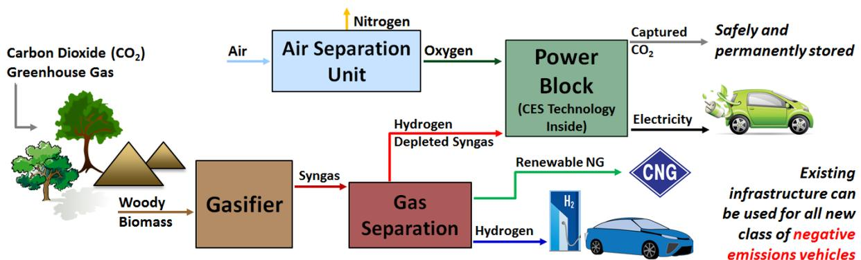
Figure 1: Simplified Schematic of CES' BioCCS Cycle
