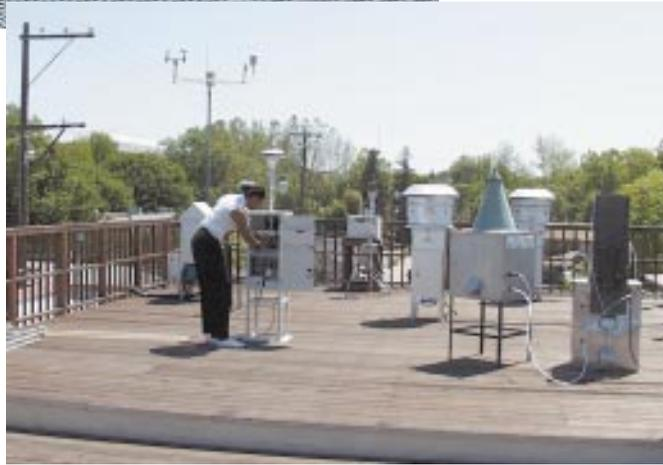
Rooftop testing station measures emissions in the air.
