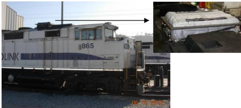
Figure 1: Compact SCR catalyst assembly installed in SCAX 865
