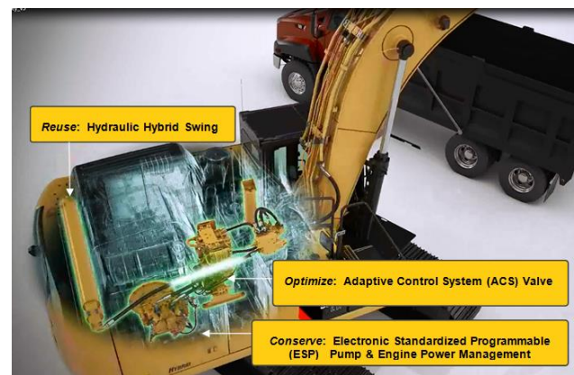
Figure 8 Cyclical Hydraulic Excavator Process
