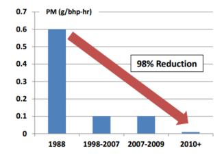
The above image demonstrates how far diesel emission control technology has come in just the past 20 years. Most amazing, is while U.S. emission standard have fallen dramatically, <u>recent testing</u> shows that the engines are actually outperforming the standards by a wide margin.
