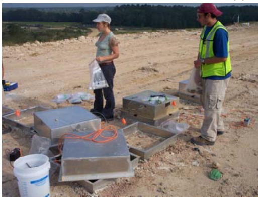
Figure 6. Students from Florida State University carried out chamber based flux measurements.
