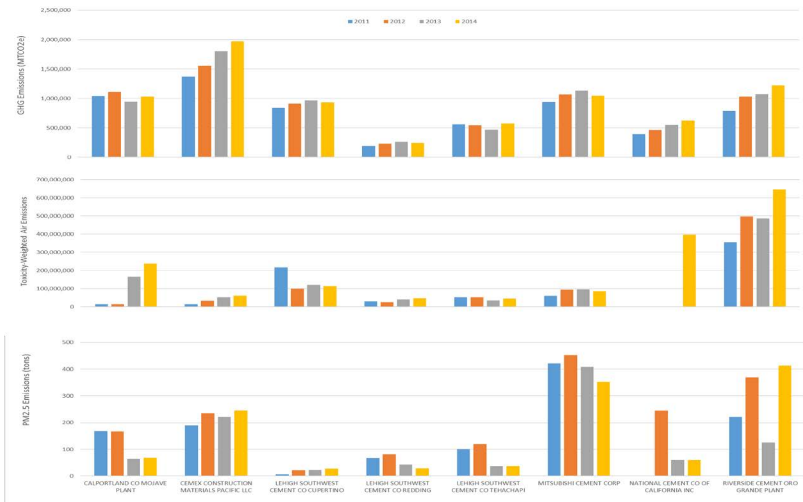
Figure 7. Cement Plants: Emitter Covered Emissions of GHGs (MTCO 2 e, MRR Data) (Top), Toxicity-Weight Air Emissions (TRI Data) (Middle) and PM 2.5 Emissions (in tons, CEIDARS Data) (Bottom) over the Years 2011-2014.
