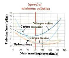
A new transmission lets you keep the motor running at constant speed, all the time, in the city and the freeway. The motor manufacturer can decide to keep his motor running, all the time, at the speed of minimum pollution. The production of NOx, CO, CO2 increases at low speed and at high speed. There is a speed where pollution is reduced to a minimum. This is where we can stay, all the time.
