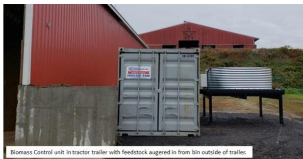
used for bedding though there can, at times, be too much material for the farm's needs. When running full time, the BR can produce roughly 1 m<sup>3</sup> of biochar per day from 5 m<sup>3</sup> of dewatered manure.
