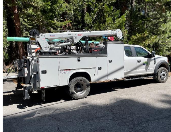
Figure 2 Class 5 Water Utility Crane Service Body
