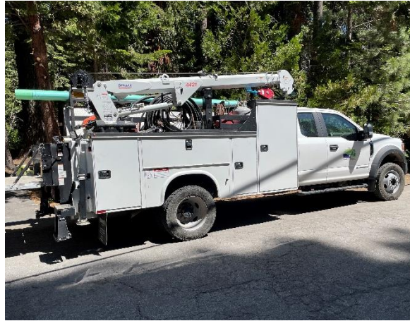
Figure 2 Class 5 Water Utility Crane Service Body
