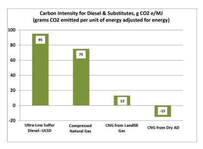
Renewable CNG From Anaerobic Digestion Is Carbon Negative
