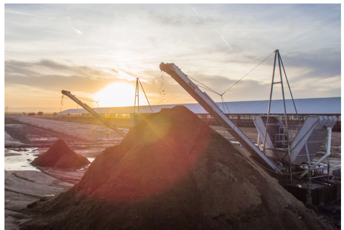
Figure 9. Manure solid separator, climate-smart dairy project on a California dairy farm.
