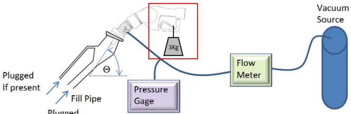
Figure B: Set-up of Testing Equipment
