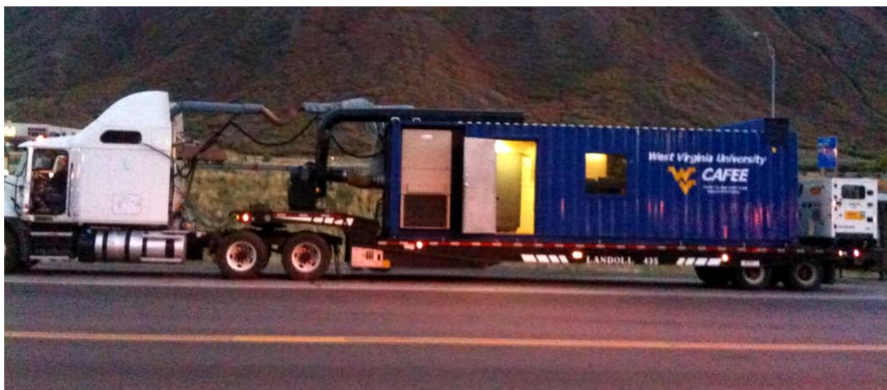
Figure 11 WVU TEMS performing real-world emissions testing
