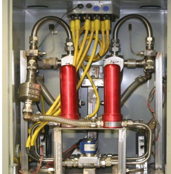
Figure 13 40 CFR Part 1065 compliant PM sampling system on-board the WVU TEMS
