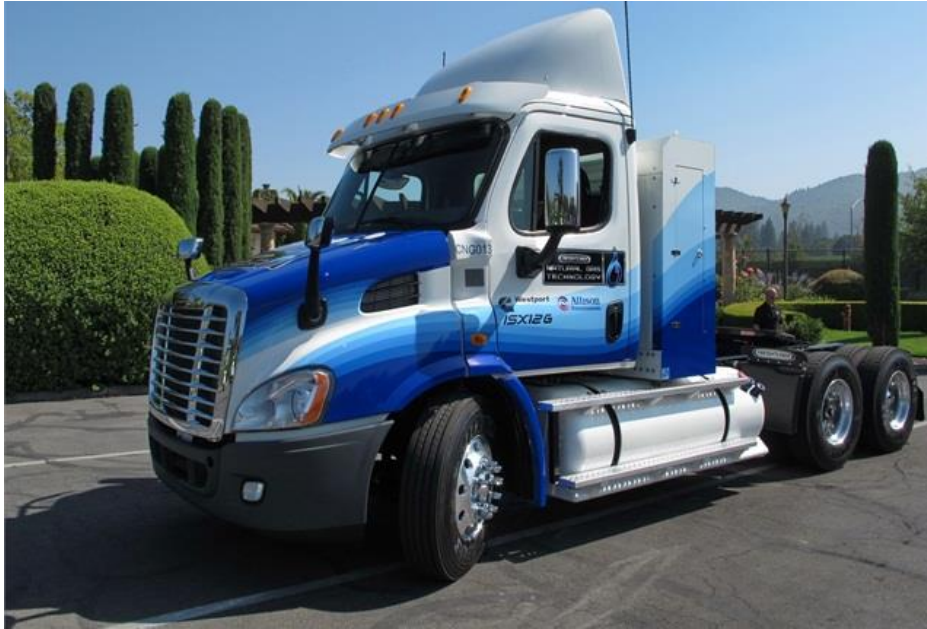
Figure 16: CNG tanks mounted behind the cab – Source: Freightliner
