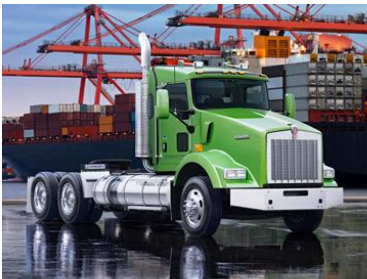
Figure 17: Typical LNG framerail tank placement – Source: Kenworth Trucks
