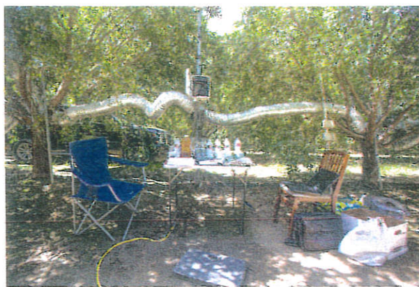
Exhaust from a propane generator and several vehicles is collected and fans funnel it through a system of ducts. The cooling system uses water from a children's pool, a pump, a sprinkler and a condenser. Photo credit: The Bakersfield Californian; Eliza Green
