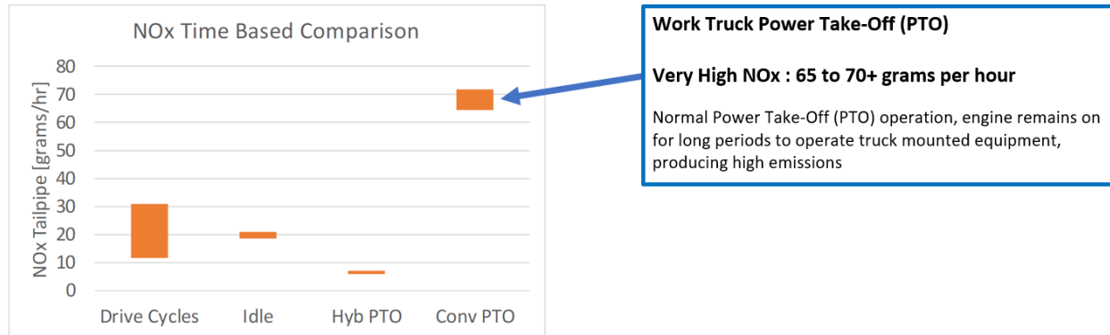
Figure 54. Time-based NO x emissions for the various operating modes
