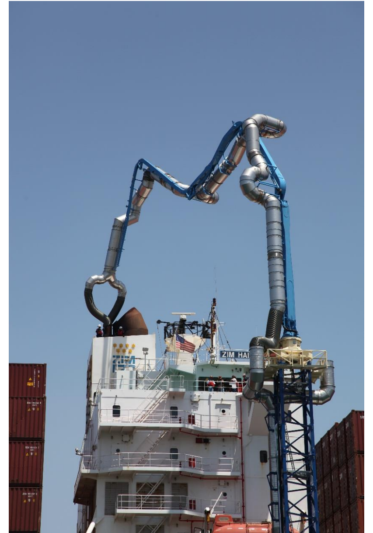
AMECS Barge System At-Dock Direct-Connect Stack Exhaust Capture System
