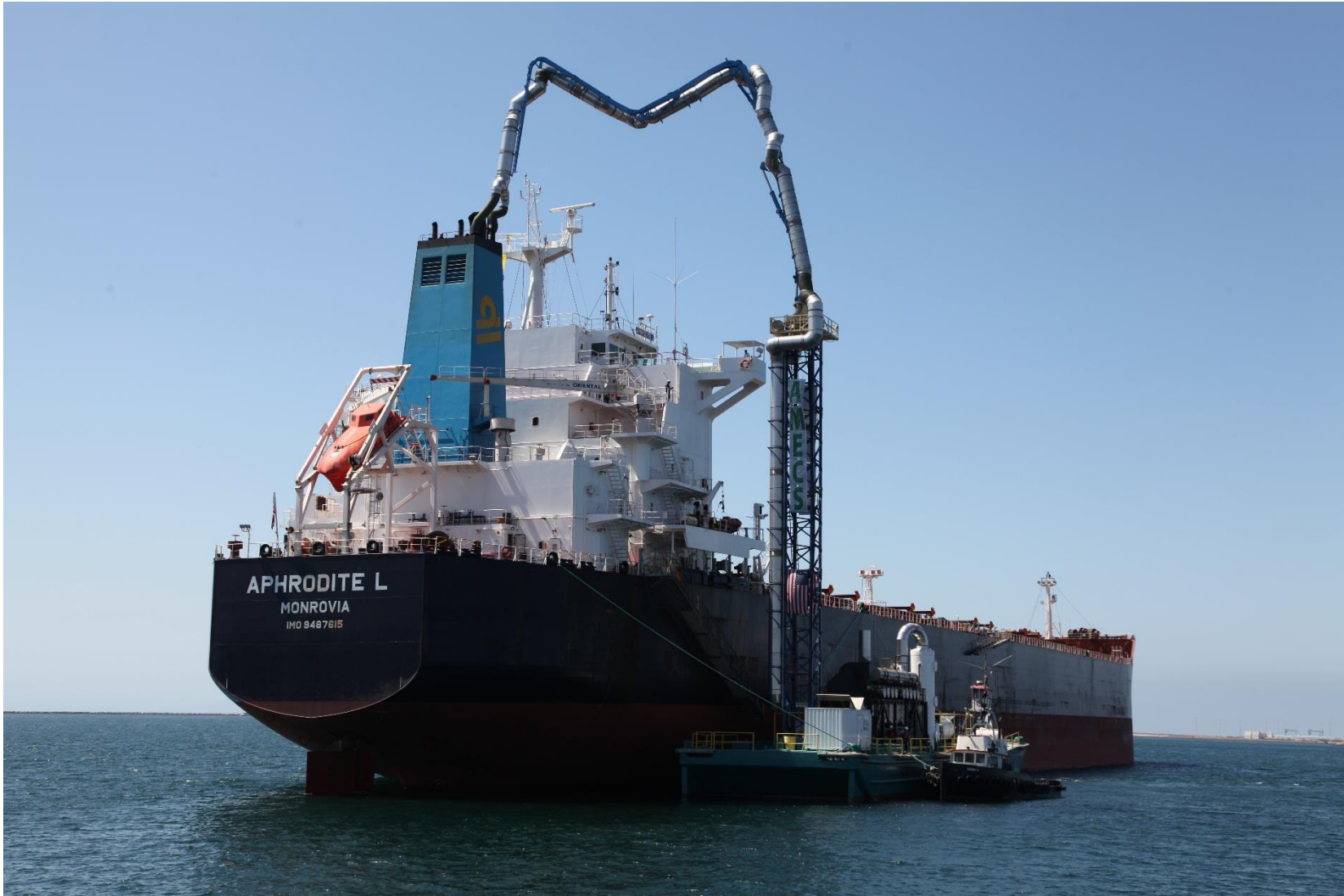
AMECS Barge System At-Anchor Direct-Connect Stack Exhaust Capture System
