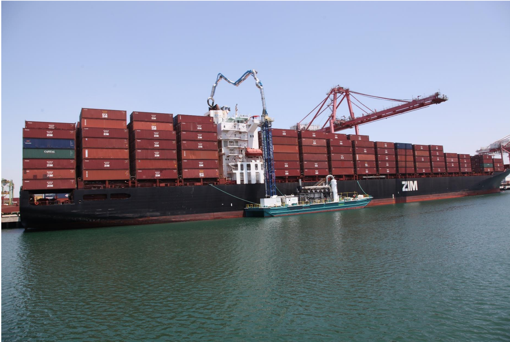
AMECS Barge System At-Dock Direct-Connect Stack Exhaust Capture System
