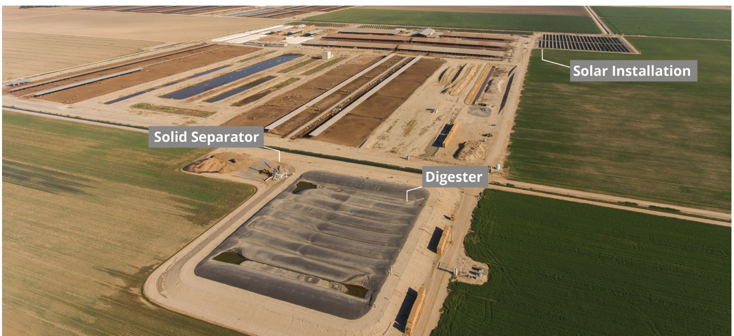
Figure 10. California climate-smart dairy with a digester, manure solid separator, and solar installation.
