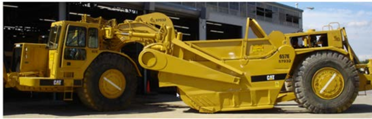
657 Scraper, unregulated to Tier 4 (dual engine)
