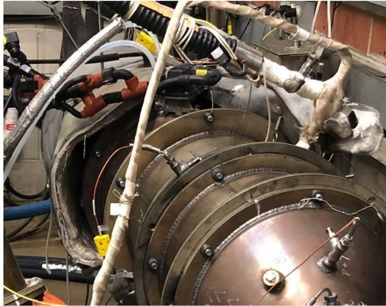
**FIGURE 13. PRODUCTION CUMMINS DEF DOSER INSTALLED ON TEAM 2 DOWNSTREAM UNIT**
