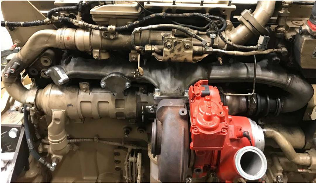
**FIGURE 24. AGI EXHAUST MANIFOLD INSTALLED ON STAGE 3 ENGINE**
