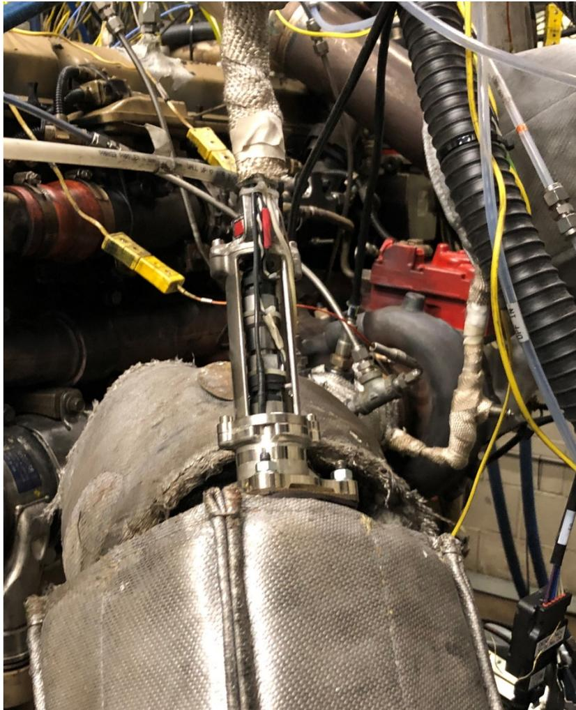
**FIGURE 12. TEAM 2 HEATED DOSING SYSTEM HARDWARE INSTALLED AT IN-PIPE LOCATION (USED FOR CONFIGURATION 2B)**
