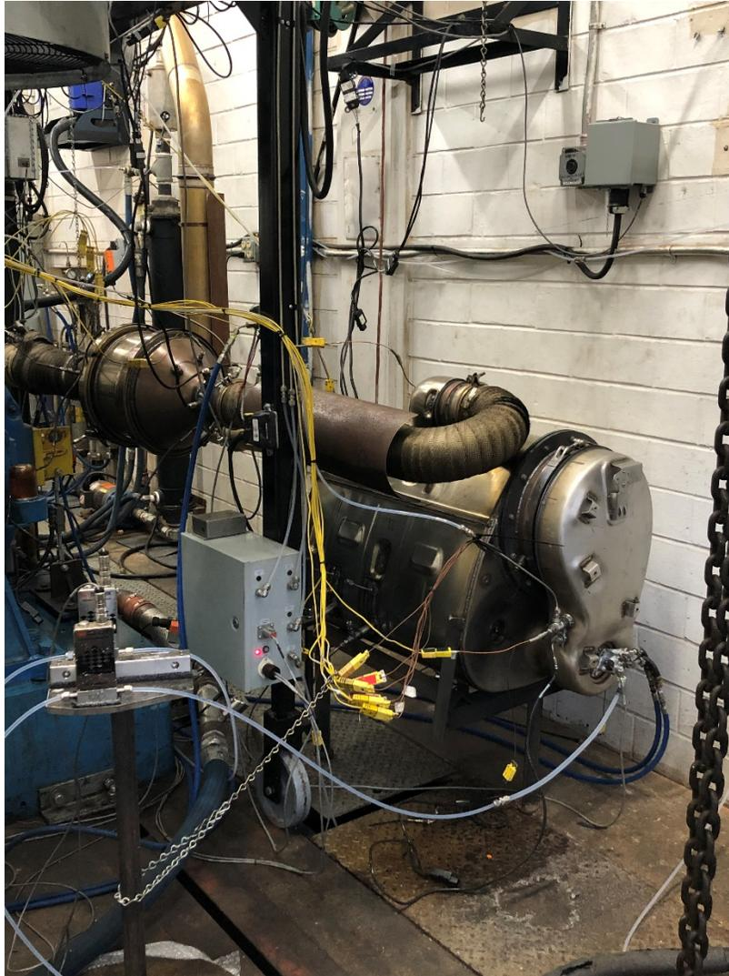
**FIGURE 56. STAGE 3 AT SYSTEM INSTALLED IN DAAAC AGING CELL**
