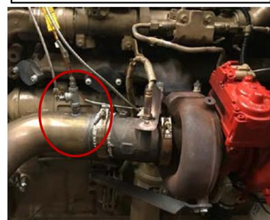
**FIGURE 25. PRESSURE AND TEMPERATURE MEASUREMENT LOCATIONS ON STOCK AND AGI EXHAUST MANIFOLDS**
