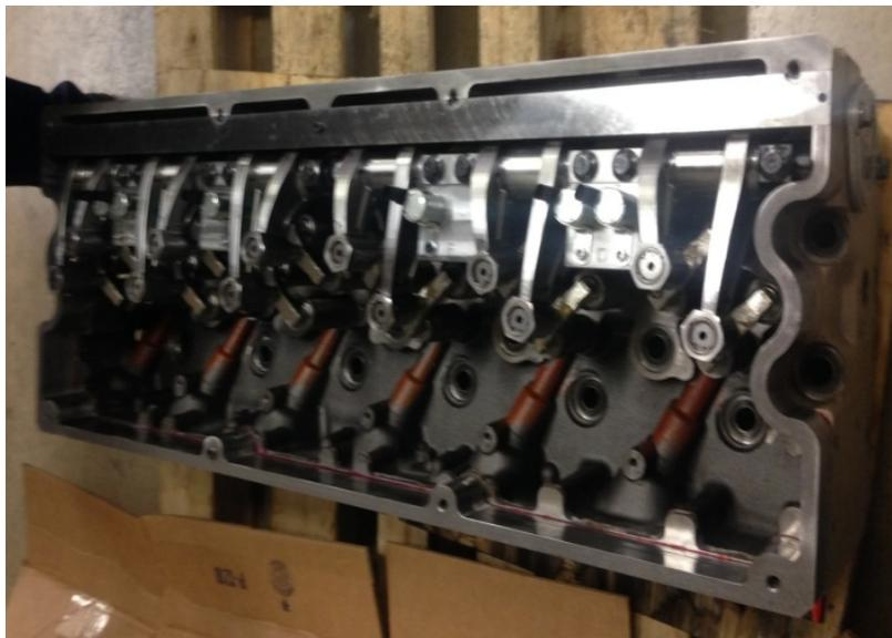
**FIGURE 32. X15 CYLINDER HEAD SHOWN WITH CDA HARDWARE INSTALLED FOR ALL SIX CYLINDERS**
