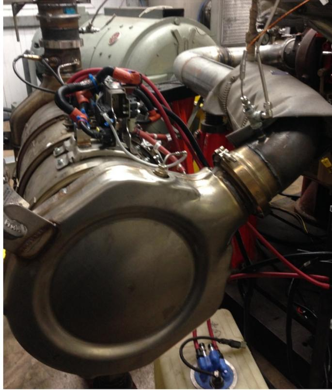
**FIGURE 4. BASELINE (STOCK) AFTERTREATMENT (INLET SIDE) FOR 2017 CUMMINS X15 ENGINE**
