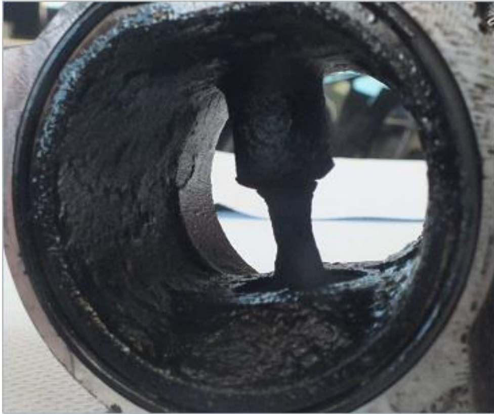
Figure 6 Disassembled EGR valve with carbon deposits (after Phase 6)
