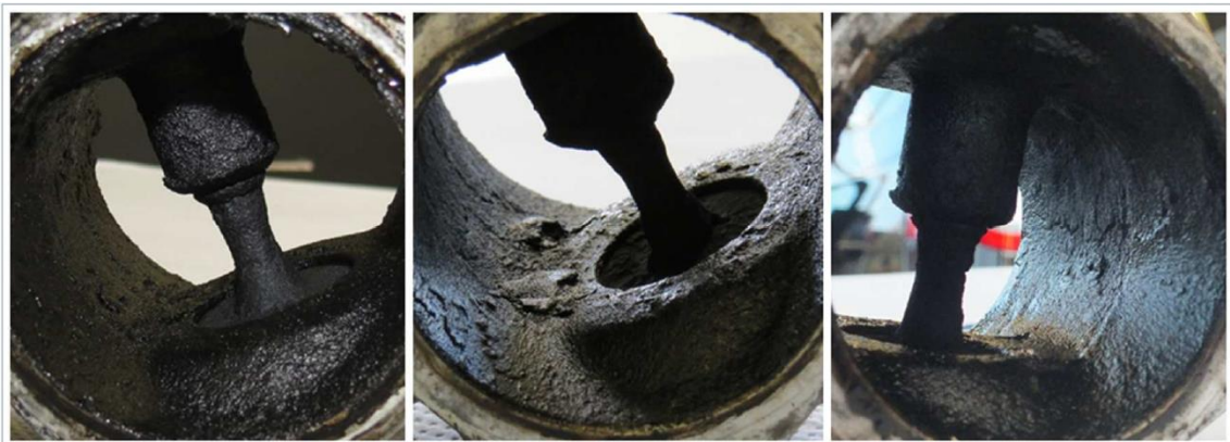
Figure 15 EGR valve in initial state, after phase 3 and in final state (left to right), view from the back
