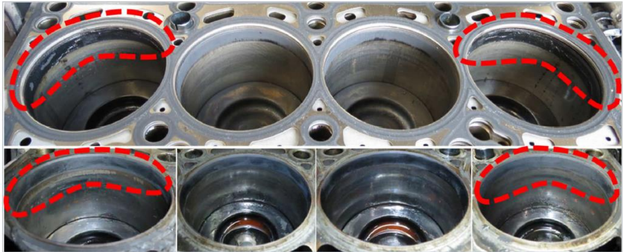
Figure 10 Cylinder bores in initial (top) and final (bottom) state
