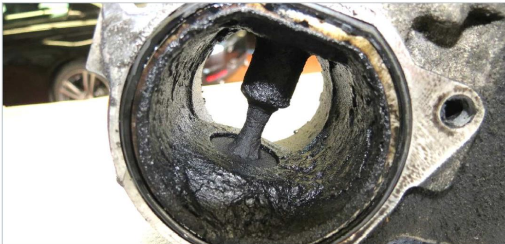
Figure 2 EGR valve with carbon deposits (initial state)
