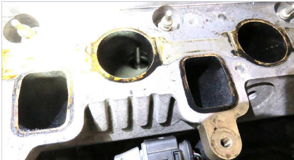
Figure 5 Intake ports of the cylinder head with carbon deposits (after Phase 3)
