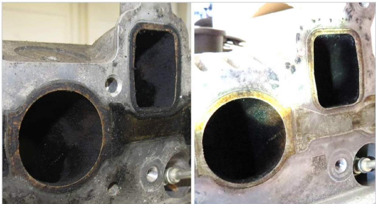
Figure 11 Intake and outlet ports in initial state (left) and final state (right)
