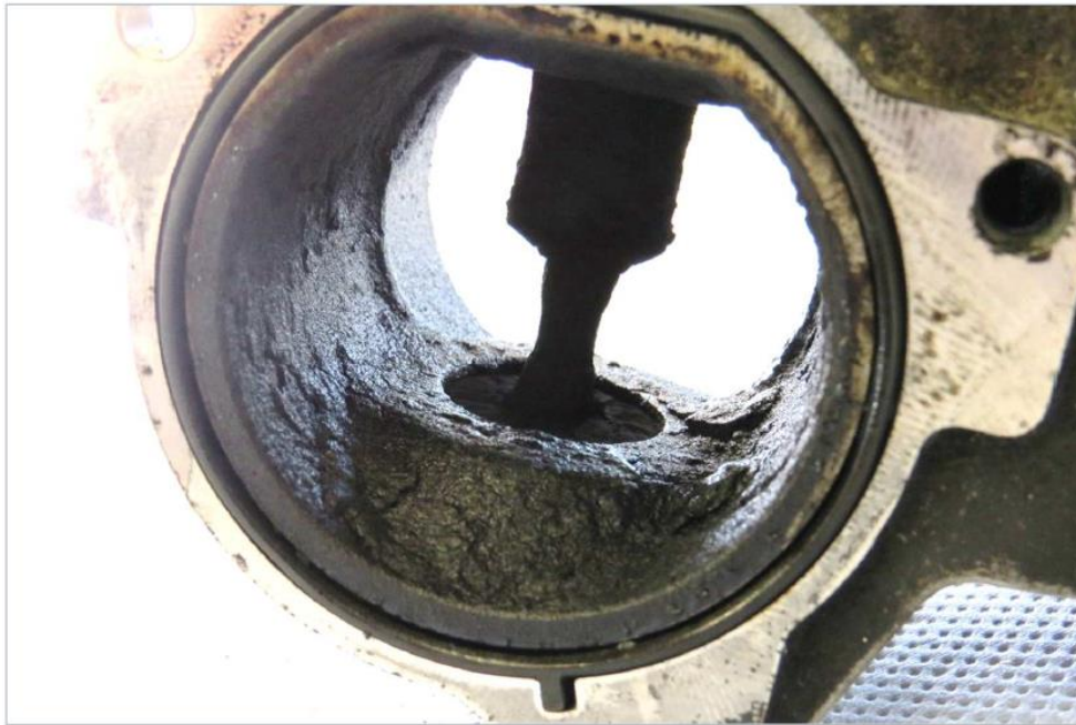
Figure 4 EGR-valve with carbon deposits (after Phase 3)
