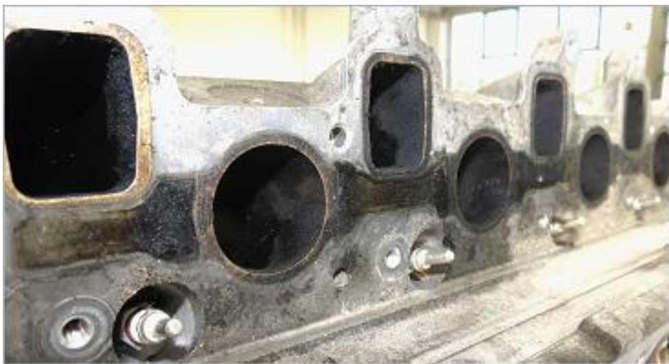
Figure 3 Intake ports of the cylinder head with carbon deposits (initial state)
