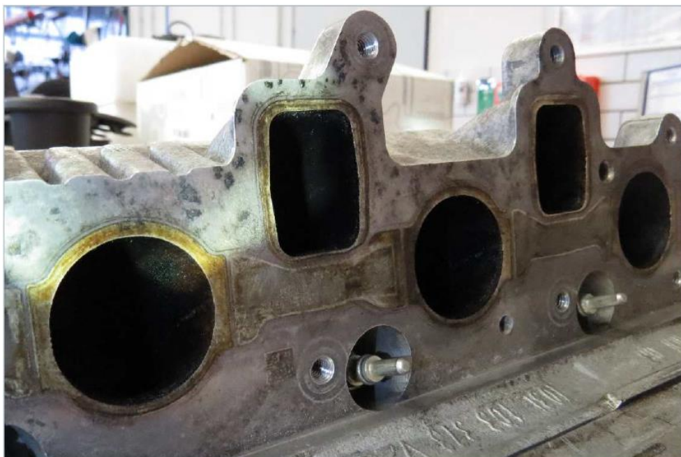
Figure 7 Intake ports of cylinder head with carbon deposits (after Phase 6)
