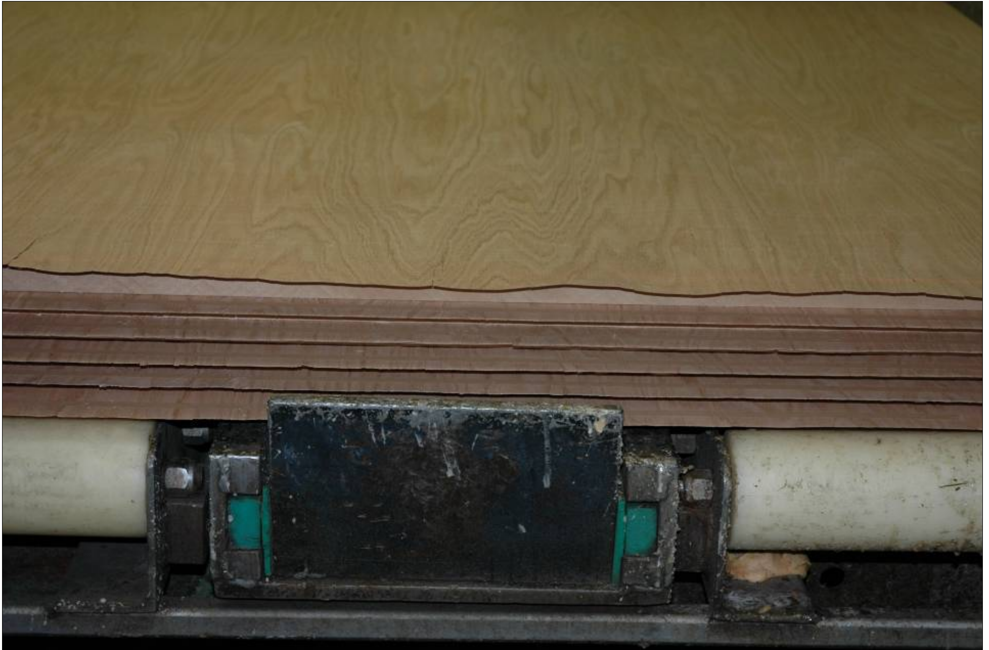
Lay up of MDF core with PVA showing oak veneers before pre-pressing
