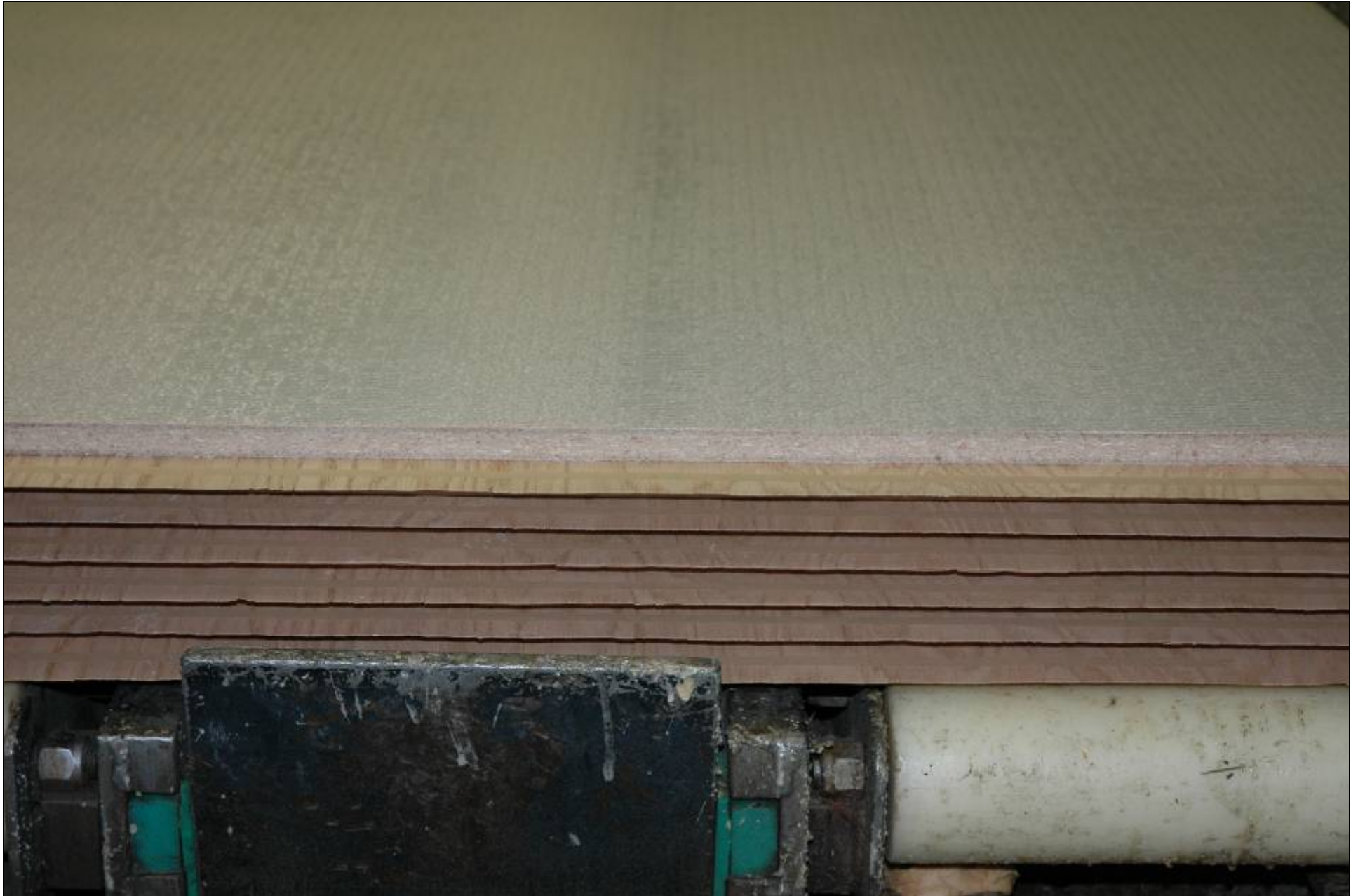
First PBC core through the spreader before the next pair of decorative veneers
