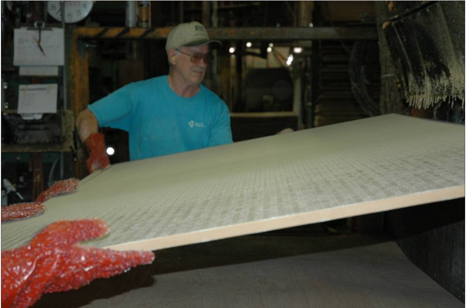
Lay up of MDF core with PVA
