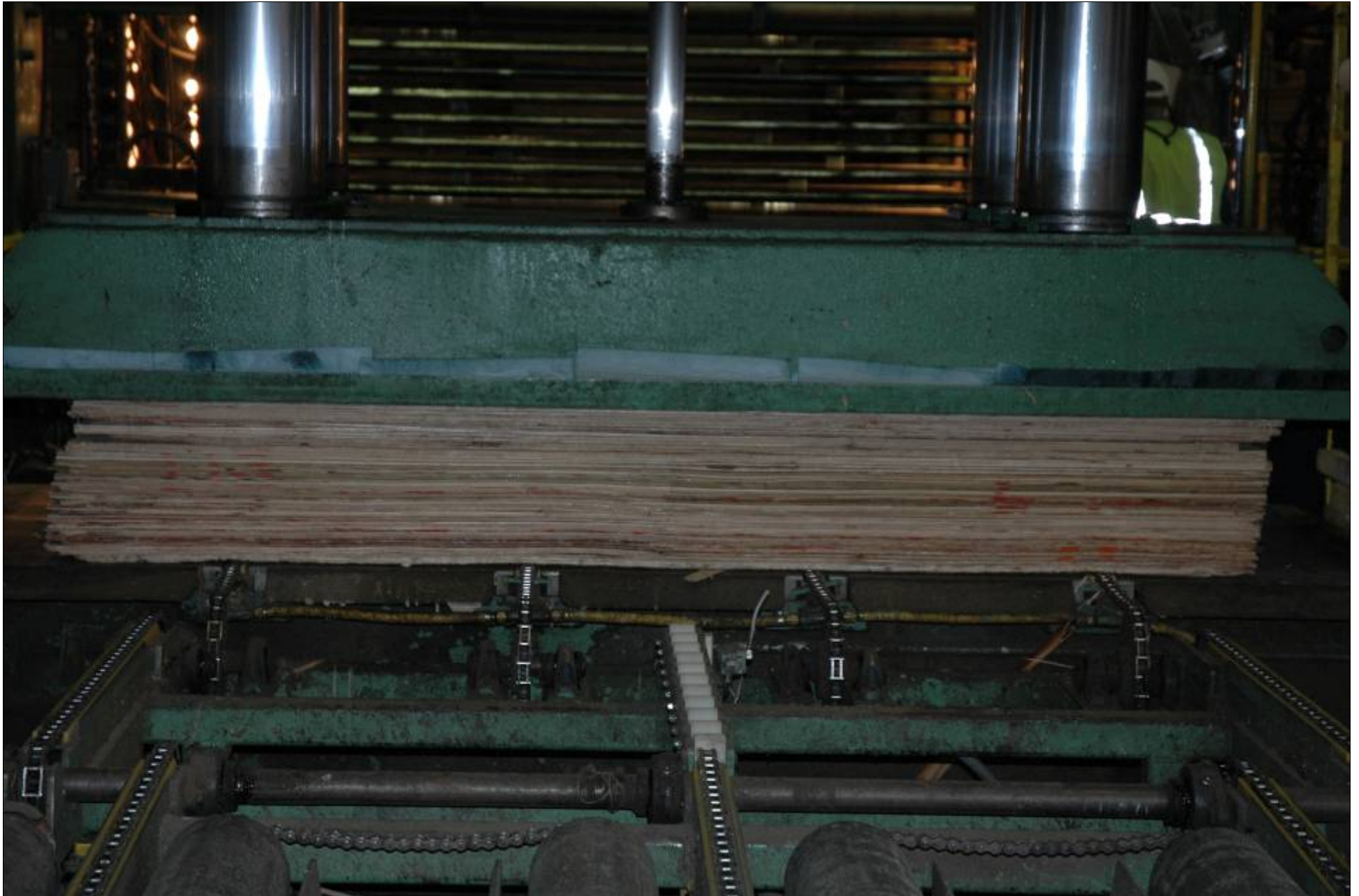
Pre Pressing VC panels to get them to tack together for loading into the hot press
