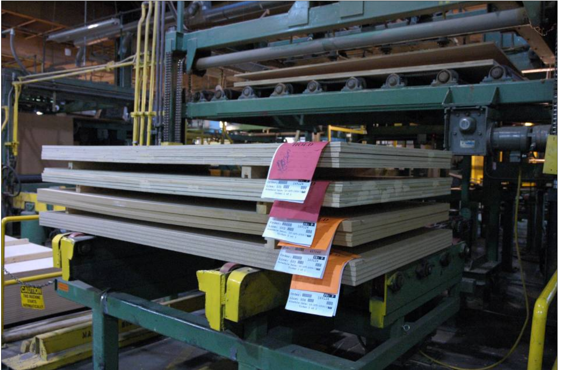
Panels ready for the sander
