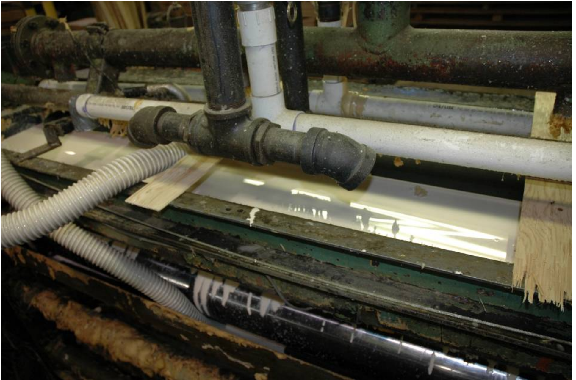
Flowing PVA into the spreader - no modifications required
