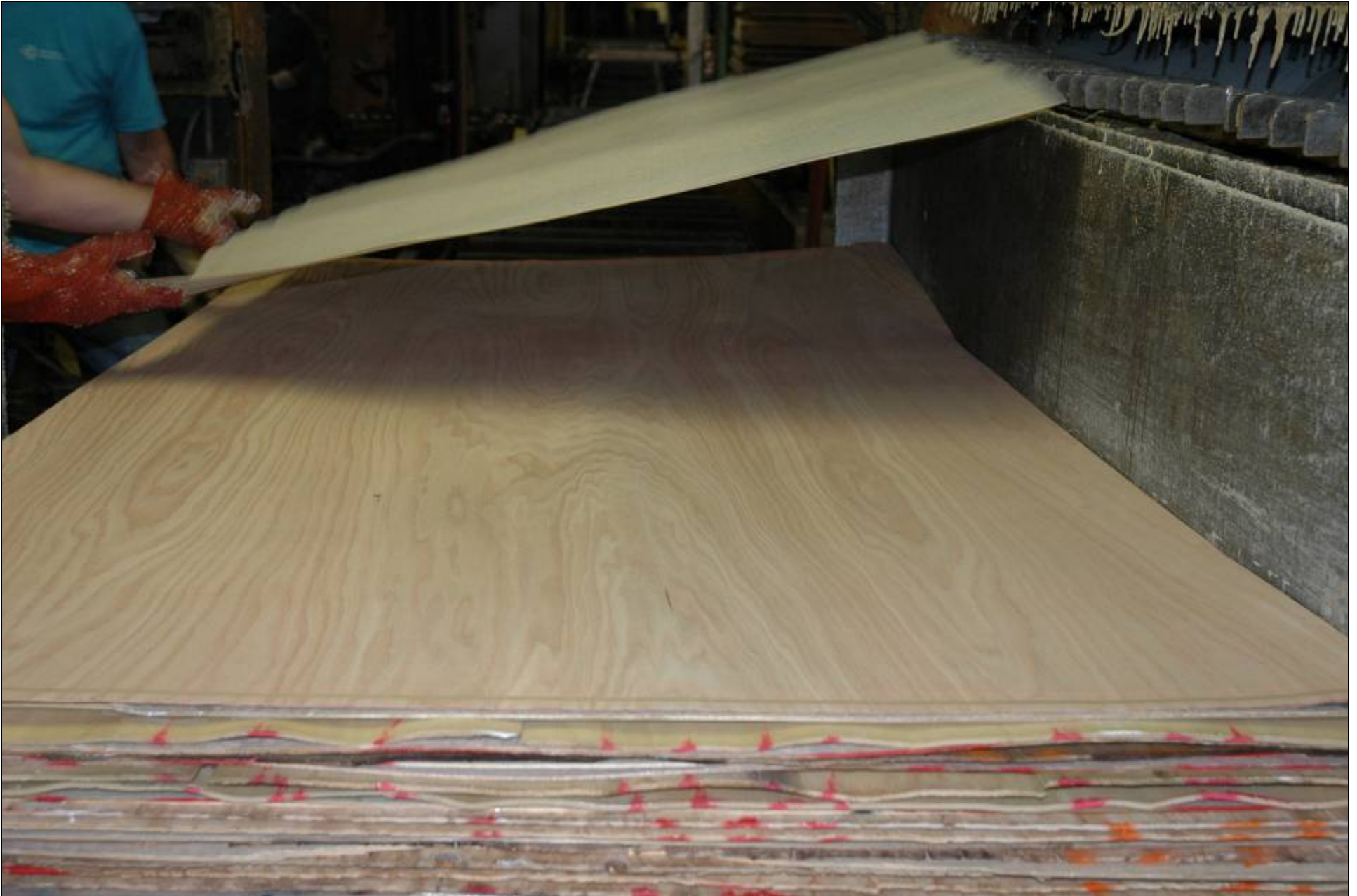
Lay up of veneer core with PVA adhesive
