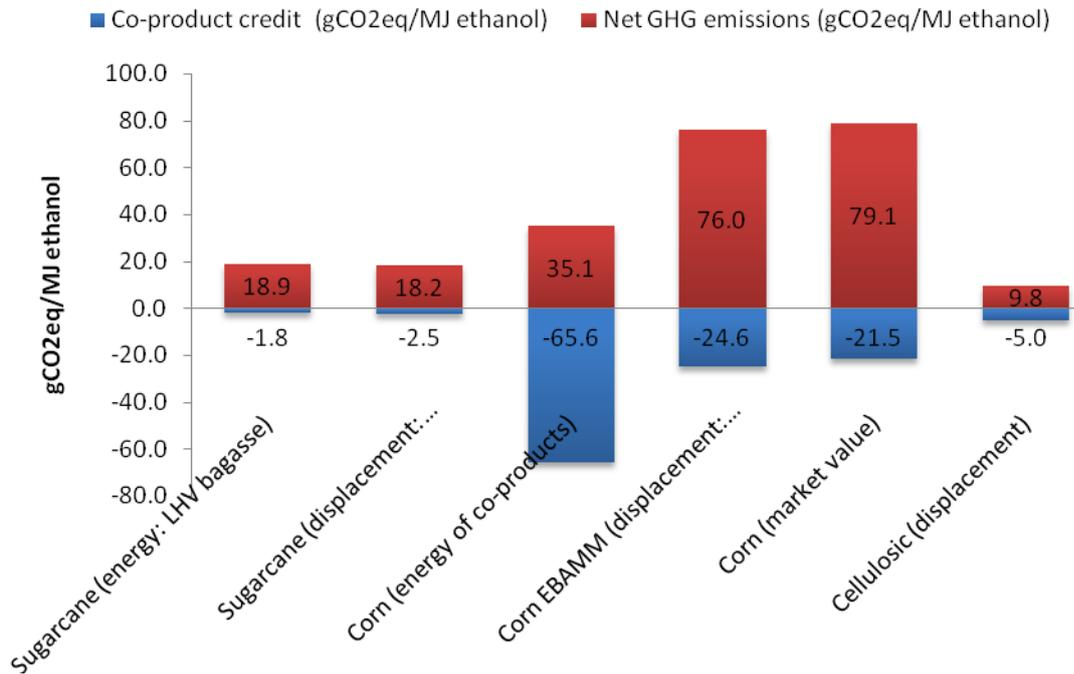
The co-product credits for biofuels (in blue) can substantially reduce the overall GHG emissions (in red) when applied.
