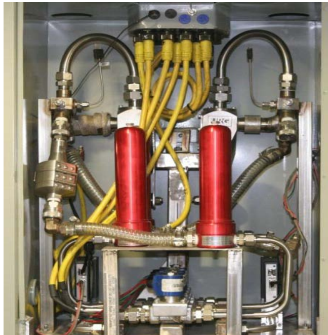
Figure 6: 1065 compliant PM sampling system on-board the transportable laboratory container
