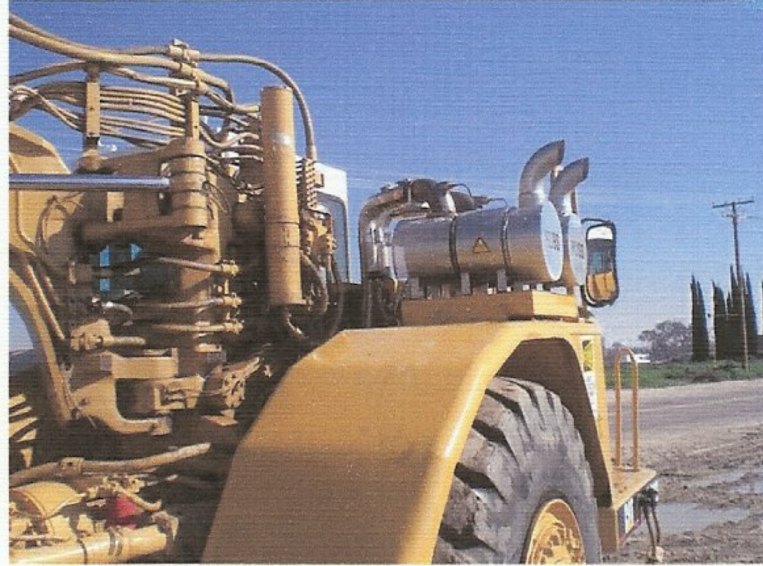
HUSS filters mounted on fender
