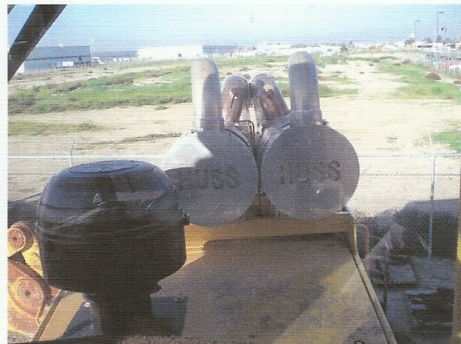
Operator's impaired view to rear of machine
