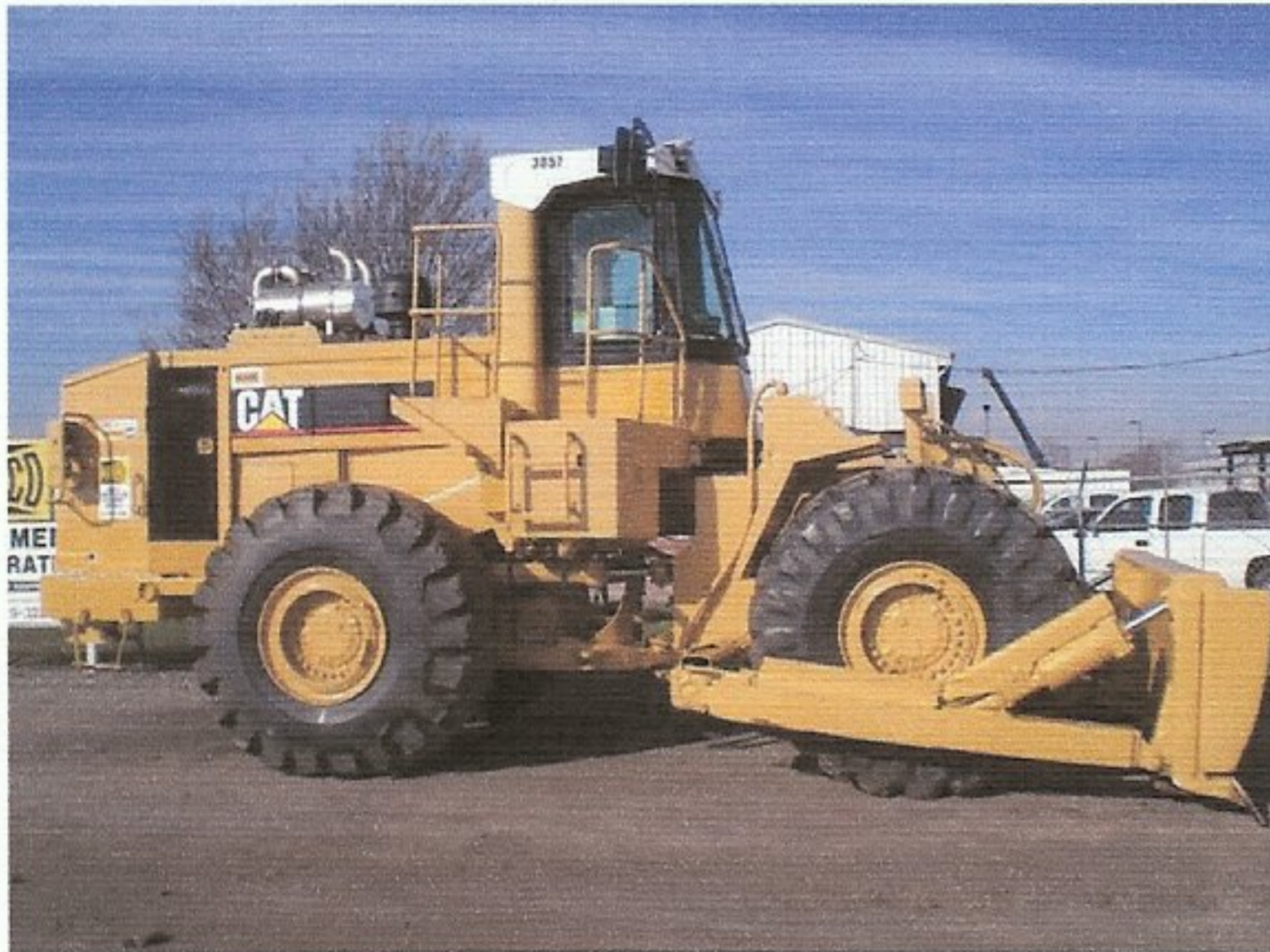
Rubber-tired dozer with HUSS filters
