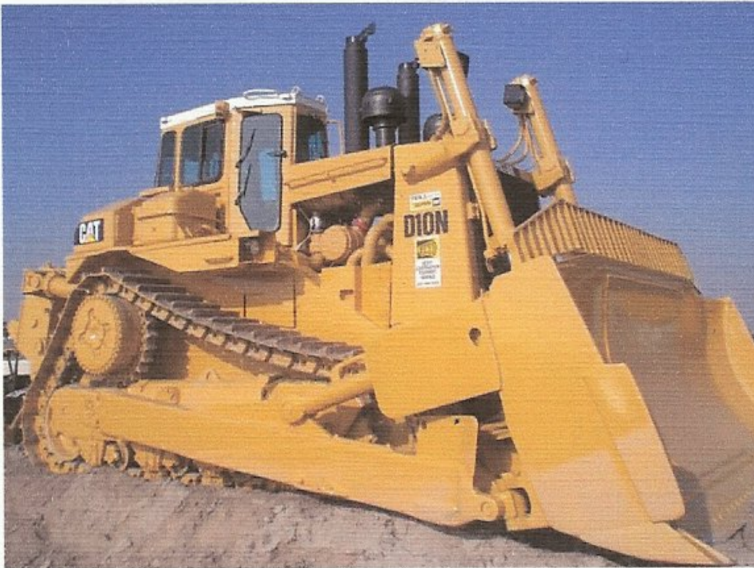
Dozer with passive Caterpillar filters installed
