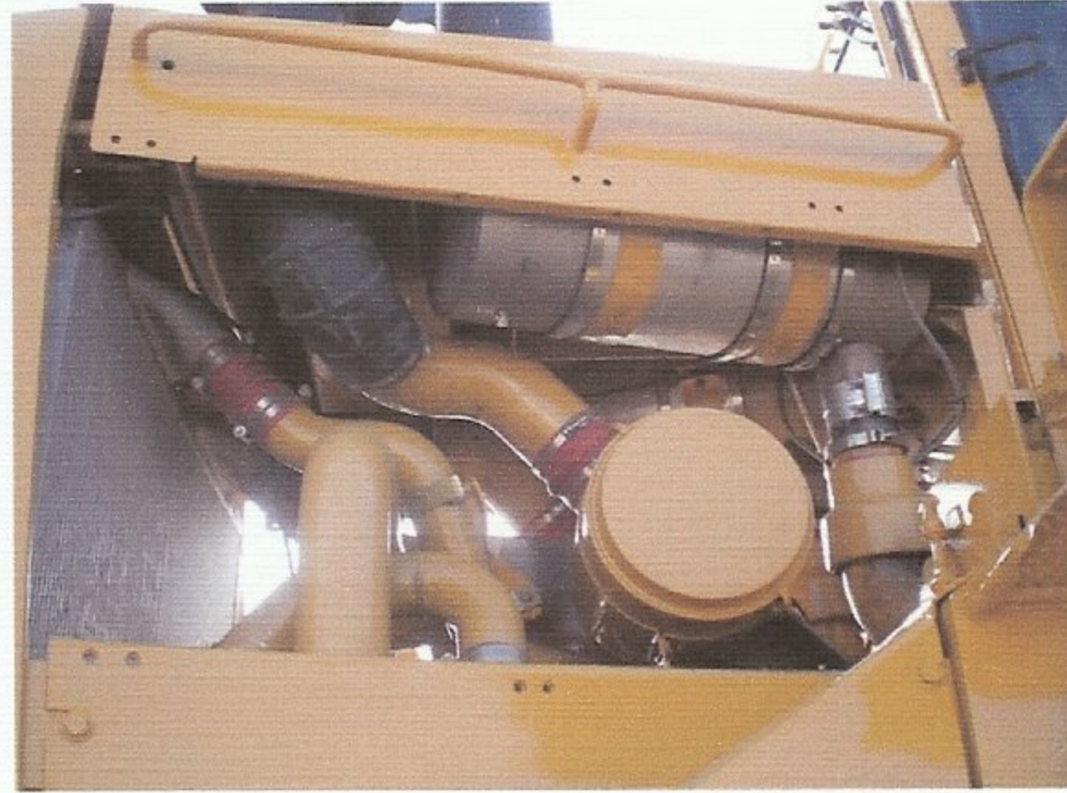
Caterpillar filters inside engine compartment
