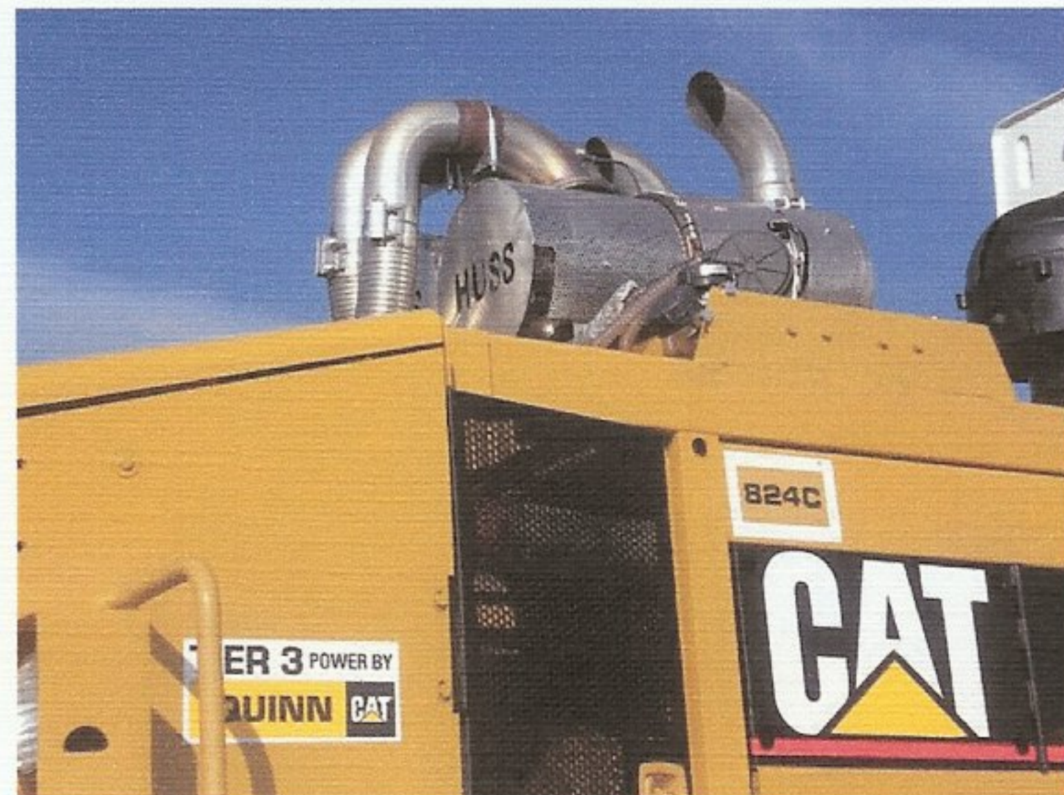
HUSS filters at rear of operator cab
