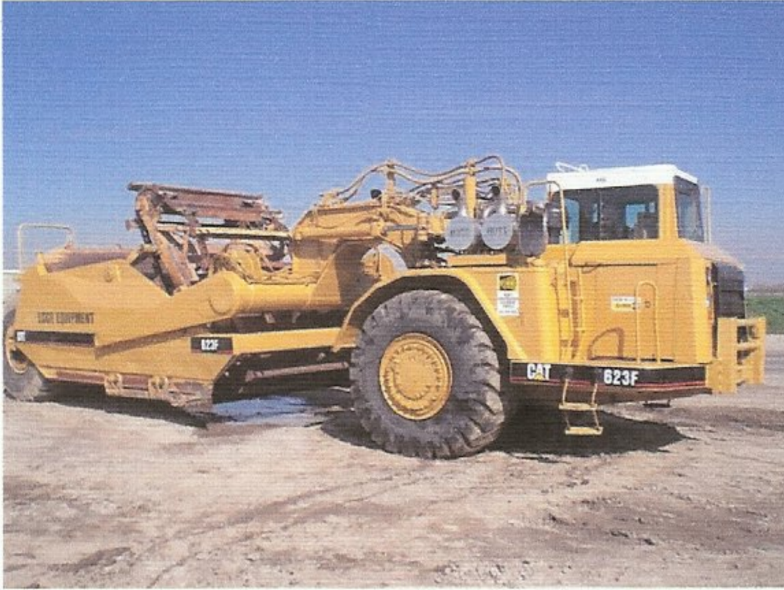
Scraper with mounted HUSS filters
