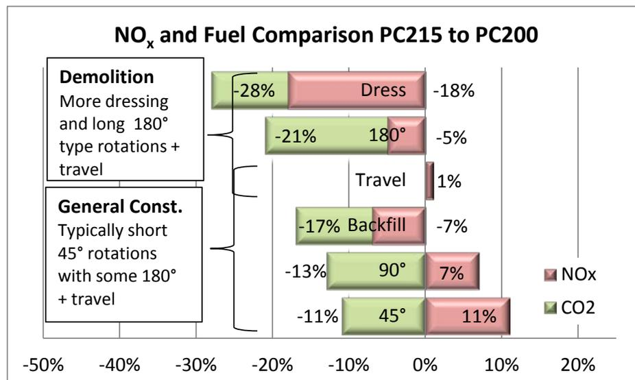
**Figure ES-9: Hybrid PC2015 NO<sub>x</sub> and FE benefit for typical excavator vocations**
