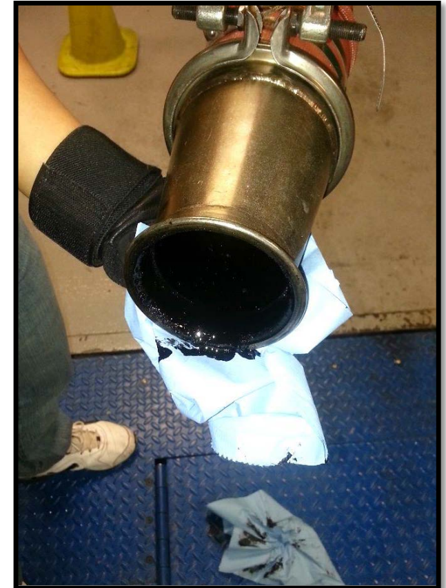
Contamination of CARB emissions lab sample train
