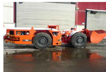
Mining Truck 64kWh dual battery -- lithium iron phosphate
