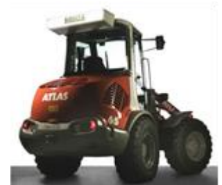
Wheel-loader hybrid 500 V Lithium force air cooled
